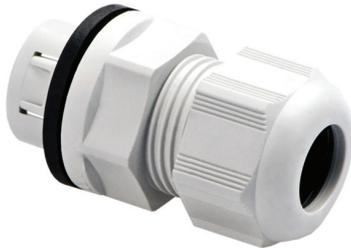
NPG, Quick-Connect™ allows for fast and effective fitting of cable glands without access to the inside of an enclosure, greatly speeding up installation.
