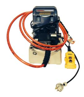
The pump produces a full 700bar (10,000psi pressure) and has sufficient oil volume to power all CABAC and MSS remote crimper heads (up to 60 Tonnes) and cutters.
