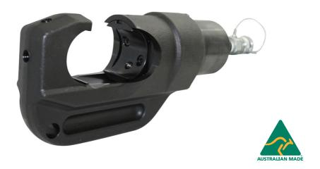
This C head style remote pump operated crimping tool develops 13 tonnes crimp force at the die faces. It has a crimp capacity of 400mm<sup>2</sup> Copper.
